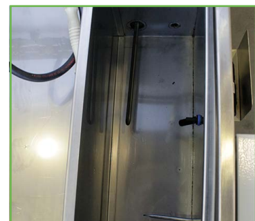
Electric heater thermostat and level shut off separated from main wash area to prevent damage and prolong life of machine.
